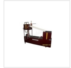
Flow Through Notches
