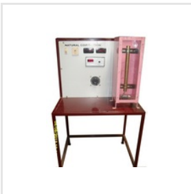
Natural Convection Apparatus
